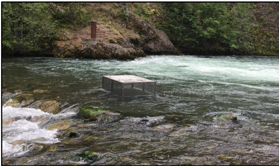
Figure 2. Stainless steel pen (0.9 m x 1.2 m x 1.8 m) used for holding Bull Trout after collection and before rapid response genetic testing and transport.
