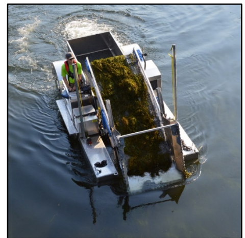
Figure 4. Harvester using the sickle cutter head. Photo Credit: BCD
